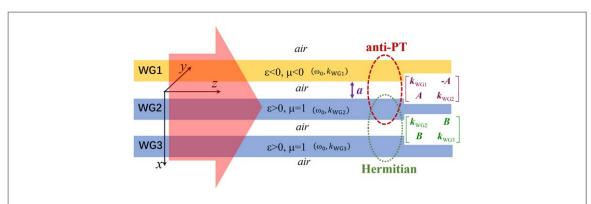
Figure 1. Schematic of the configuration under investigation, which contains three straight lossfree WGs. WG1 is made of a NIM with  $\epsilon_{\rm NIM}=-3$  and  $\mu_{\rm NIM}=-0.556$ . WG2 and WG3 are made of dielectrics.
