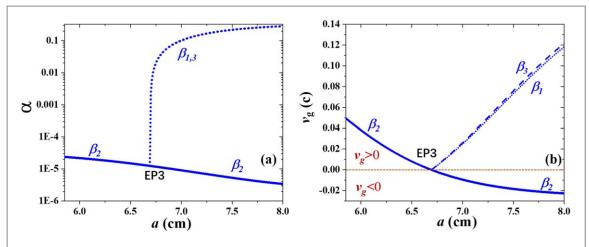
**Figure 5.** (a) Ratio of field localized inside WG2, where the y axis is plotted logarithmically. (b) Group velocities  $v_g$  of the three branches. Results about complex  $\beta$  are not shown because the associated  $\alpha$  and  $v_g$  are not well defined.
