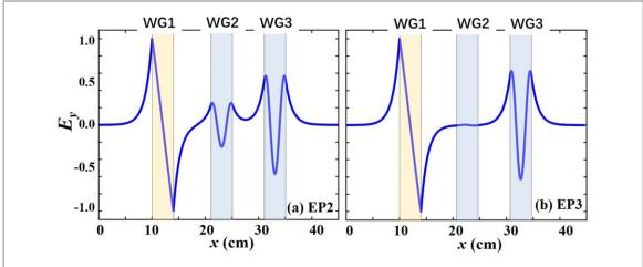
**Figure 3.** Distributions of fields  $E_y$  at (a) EP2 and (b) EP3 shown in figure 2. The fields are normalized by the maximum amplitudes in the structure.
